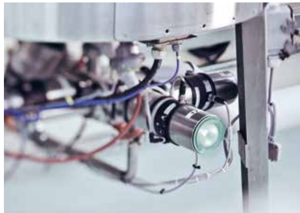
Tank bottom valve system with integrated level sensor on a preparation tank for Unither Pharmaceuticals.
